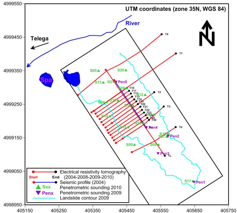
Figure 3: Location of geophysical measurements and penetrometric soundings
